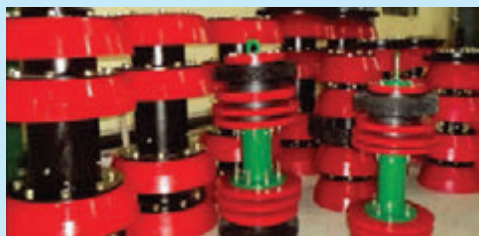
PIPELINE CLEANING PIGS
